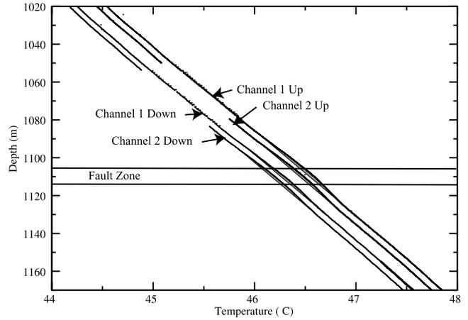
**Figure 2.** Original temperature profiles obtained near the fault zone. The shaded portions show the temperature anomaly that is a several hundredths of a degree above the geothermal gradient.
