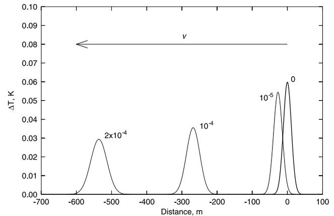
**Figure 4.** Predicted temperature anomaly including effects of water flow with flow rates of 0 (no water flow),  $10^{-5}$ ,  $10^{-4}$ , and  $2 \times 10^{-4}$  m/s.
