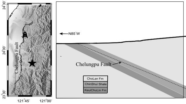
**Figure 1.** Map shows location of the drill site with respect to the surface faulting on the Chelungpu fault during the 1999 Chi-Chi earthquake. Star shows the location of the epicenter. Diagram on right shows the Taiwan Chelungpu Fault Drilling Project (TCDP) borehole that intersects the fault at 1111 m.
