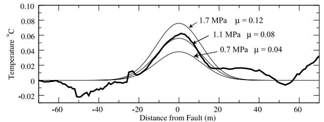
**Figure 3.** Fitting of the observed temperature anomaly (thick line) to model curves (thin lines) for a range of shear stress. The best fit values are for a shear stress of 1.1 MPa and a diffusivity of 3.4 × 10<sup>-7</sup> m<sup>2</sup>/sec.
